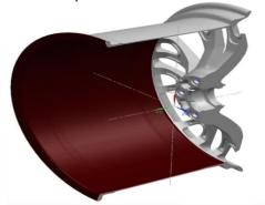
• Chrome wheels with a coated barrel (areas illustrated in red), refinishing is possible. However, the required refinishing process cannot be performed in the dealer environment. Refer to Refinisher's Responsibility
